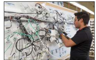
Working boards” are used to ensure the correct assembly of cables and components, as well as testing their electrical performance.
