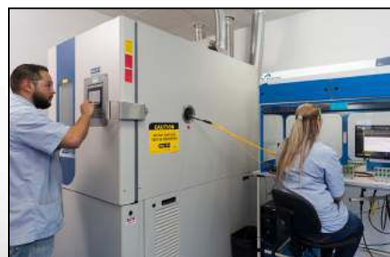
Once a prototype is made, the assembly is tested. An Environmental Chamber for temperature and humidity, along with tensile and immersion test devices, simulate demanding environmental conditions to ensure the product will perform under these stresses.
